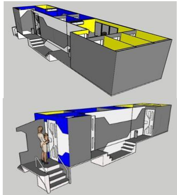
Gambar 13. Interior Mobile Toilet
