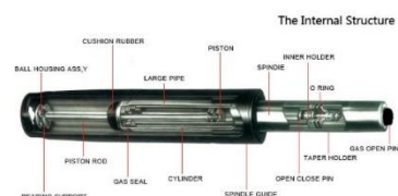
Gambar 2. 4 Struktur Gas Lift
